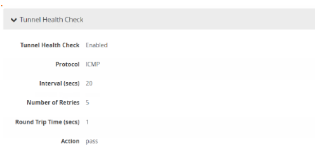
Figure 149 Configure ICMP Health Check Parameters
