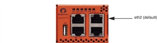
Figure 107 Stack Port Location on GigaVUE-HC1 Front
