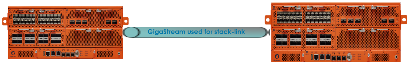
Figure 4 Daisy-Chain Configuration using GigaStream for Stack-link
